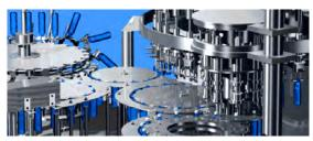
**for filling in PET-container -** water preparation, PET bottles blow molding, saturation of liquid by the carbonate acid, a blend, bottle rinsing, liquid filling, capping, labeling and shrink wrapping, overwrapping of palets by stretch film;
