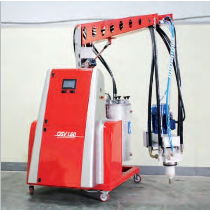
L60 has been developed in 2009 as high capacity mixing foaming machine for manufacturing facade decoration and architecture pieces from rigid PU foams. But soon it's application area has been covered almost all traditional PU foam applications such as construction panels, furniture, insulation, etc.
