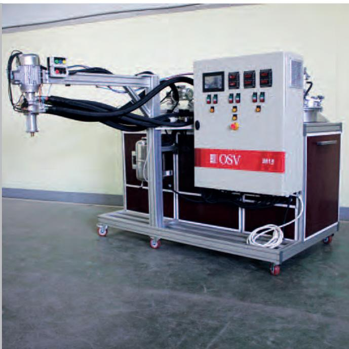
M15 is from the range of machines for processing of both MDI and TDI high performance polyurethane elastomers. Available in two and three components version it allows to work with almost all grades of hot casted polyurethanes.
