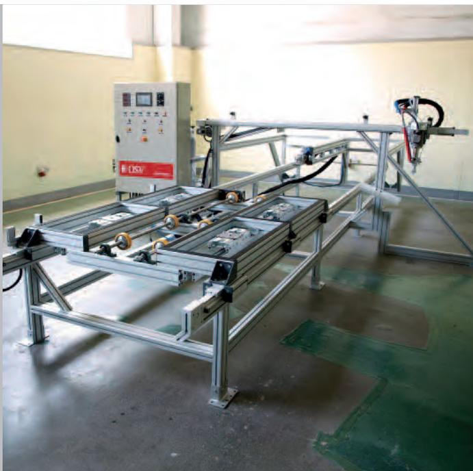
L3000 is a multi-task production line, which provides solution for three things — metal sheets, pipes, and rolls lining. Originally it has been developed for repairing of seeds transferring system but some next applications were in other industries such as printing rolls, water transferring, mining industry, etc.
